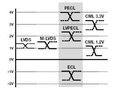
'CML numbers are shown for an 800mV output example; 400mV is also common.
